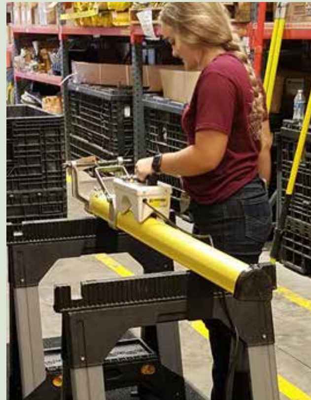
Intern Emily Gauthier tested over 685 hot arms, hot sticks and grounds this summer.
