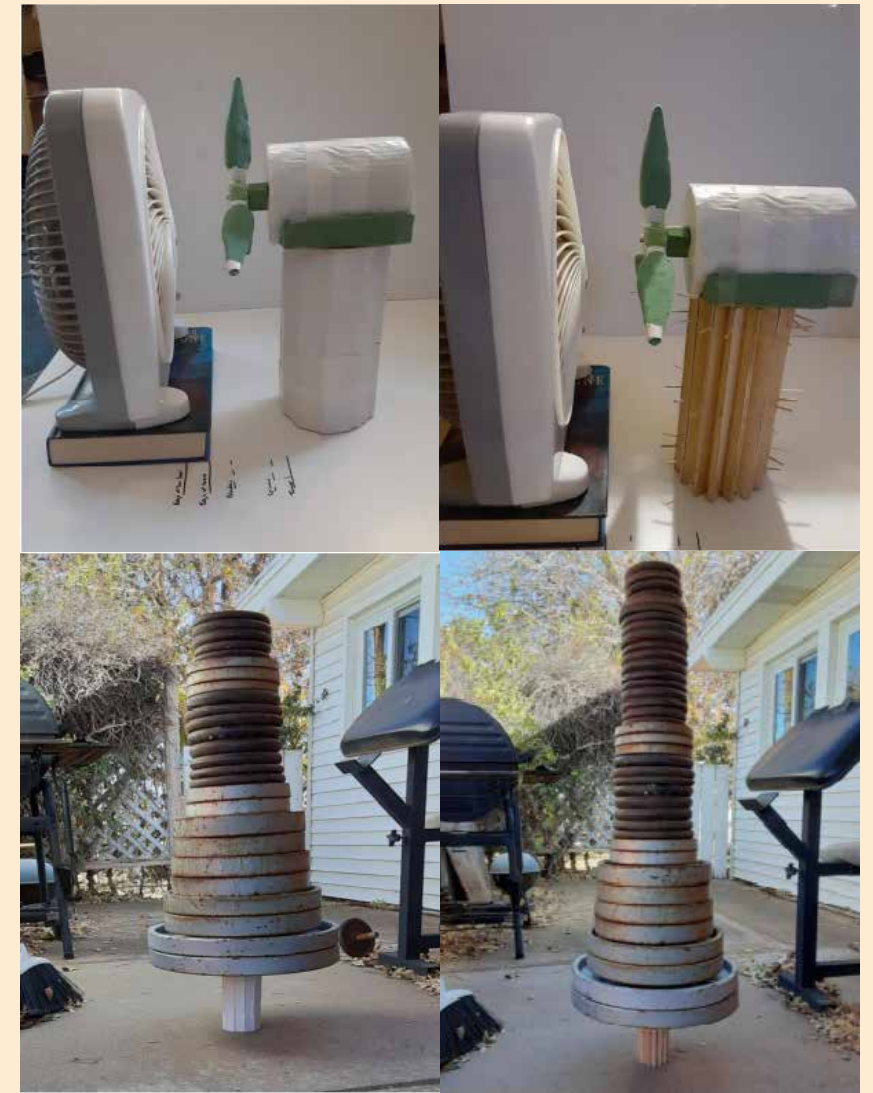
Amanda Whalen showed in pictures how she compared a standard, tubular tower as her control against a tower with pleats and spines like that of a saguaro. The saguaro-shaped tower directed more wind to the turbine and held 452 pounds compared to 400 pounds held by the control tower.
